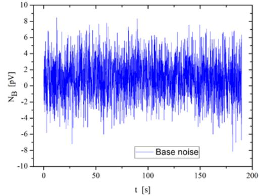
Fig. 5. IDCSD base noise, around 16 pV<sub>pp</sub>.
