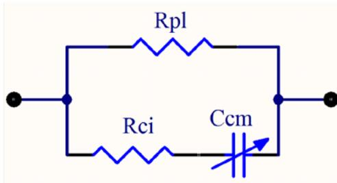
Fig. 8. Equivalent electric circuit of whole blood.
